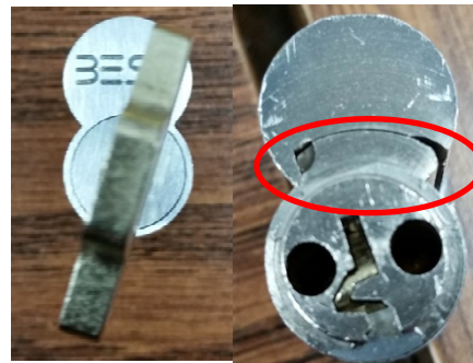
Picture 4: Left is front when key is turned; right is back when key is turned (circled area is what moves for best brand)
